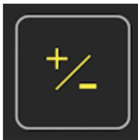
Inverts the current position. I.e. multiplies it by -1, so positive position becomes a negative position and vice versa. This function is used to move to a position that is at the same distance on the other side of the zero point. In other words, to machine symmetrical features.
