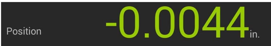
The position digits represent the current axis position. Note it takes into accounts the selected units and coordinate system (absolute or incremental). A quick select of the digits will bring up the Axis Details menu and a long touch brings up the Set Dimensions menu.
