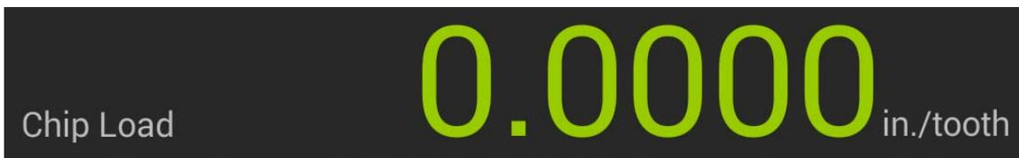
Displays the chip load when the axis is in motion and a tool has been selected. The value is calculated by dividing the feed rate by the product of RPM\* and tooth count. When no tool is selected and/or the tachometer is disabled, the display will be disabled and a toast will briefly appear informing the user that one of the above requirements is not met.
