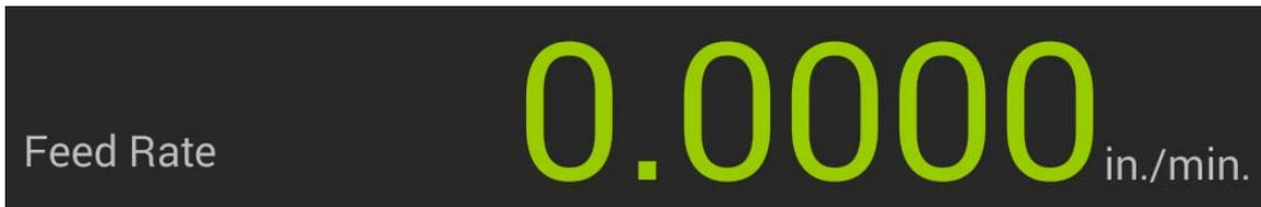
This displays the current feed rate when the axis is in motion. The value can be either positive or negative, depending on the direction of travel. The value is refreshed at a 2Hz frequency (two times per second) regardless of the velocity.
