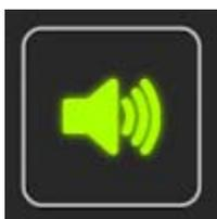
Toggles audible "near zero" alert for the current axis on and off. When selected, the DRO will emit a series of beeps starting at 0.250" (10mm when in metric mode). At 0.100"/5mm, 0.010"/2.5mm and 0.005"/0.1mm the frequency of beeps will increase. When the axis moves to within 0.001"/0.05mm of 0.000, the application will emit one 2-second long beep and stop. The alert is in effect as long as the dialog is open. When the dialog is dismissed, the alert will be turned off.
