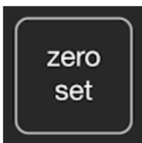
Similar to the zero set function on the main DRO screen but acts upon the selected axis only. Short pressing the button sets incremental origin to zero for the selected axis. Long pressing the button sets the work piece origin to zero for the selected axis.
